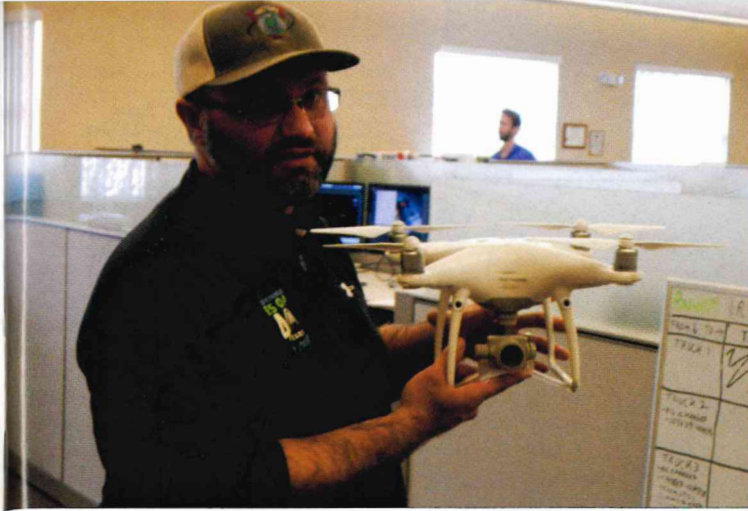
Cory Westholms shows a drone that is used to help produce a topographical scan of projects.
