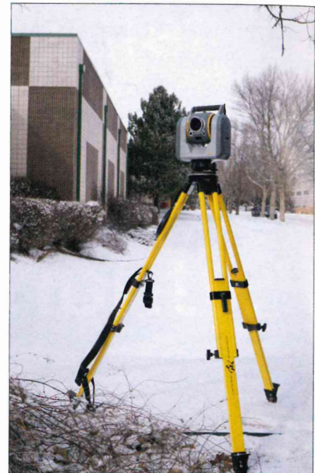
A robotic scanner can shorten surveying time and increase accuracy.
